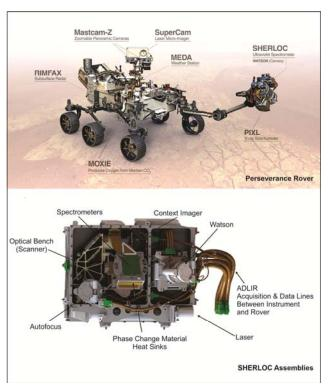
**Figure**: Perseverance rover with Scanning Habitable Environments with Raman & Luminescence for Organics & Chemicals (SHERLOC)
